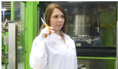
**Fiskars personnel** gives the final seal of approval to each pair of Fiskars scissors manufactured at the Billnäs factory in Finland. This is done by cutting a piece of cloth and listening to the sound of the opening and closing of the blades.
